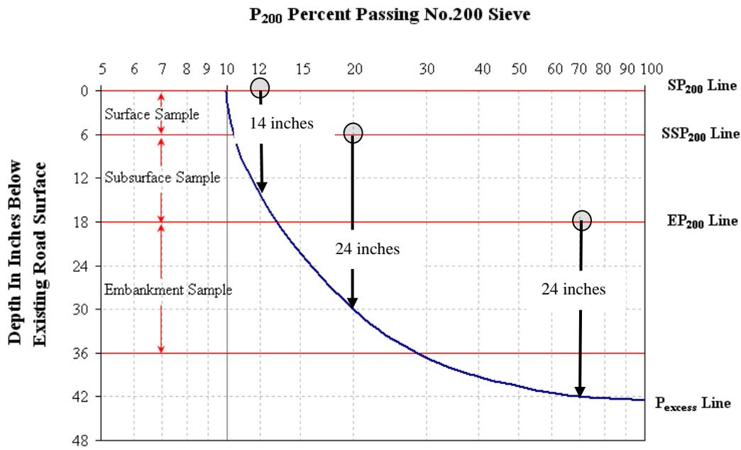
**Figure 1. Simplified Excess Fines Design Method**
