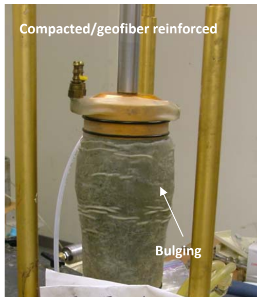
Figure 28: Failure mechanisms of unimproved and improved soil samples.
