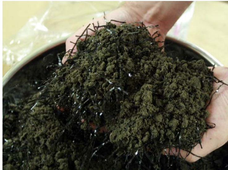
Figure 1: Sample mixture of soil, water, and geofibers.
