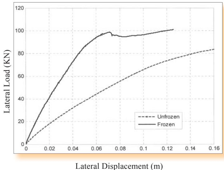
Figure 2. Lateral load vs. lateral deflection for steel pipe pile under unfrozen and seasonally frozen soils. Graph by Z. Yang.
