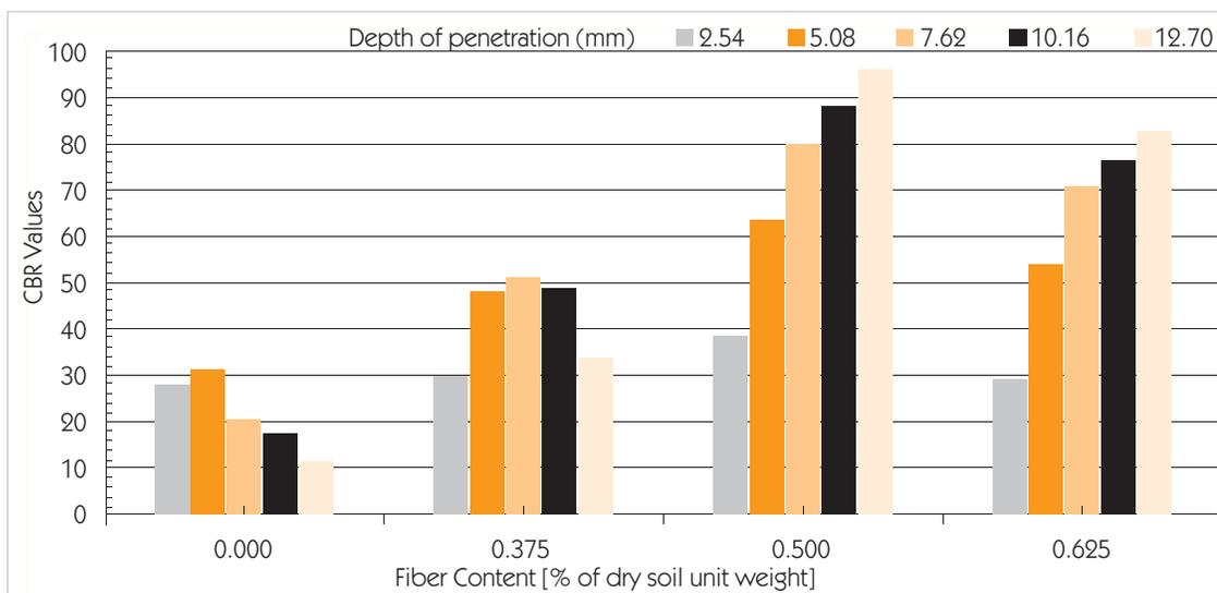
Figure 1 (left). CBR value vs. percent fiber for each depth of penetration at 11% moisture content. Graph produced by K. Hazirbaba.
