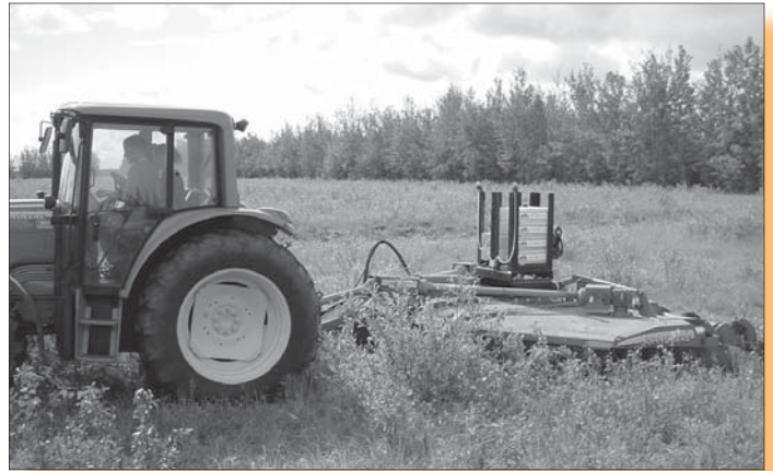
Wetblade mower cutting vegetation and applying herbicide simultaneously at the Delta Junction, Alaska field site. Photo by Daniel Debord.
